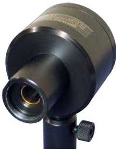
The final photo shows the THZ-WC-13 mounted on the THZ1.5B probe but with the window and aperture plate removed. This set up would result in the largest unrestricted input aperture (i.e. 13 mm) and highest optical gain.
