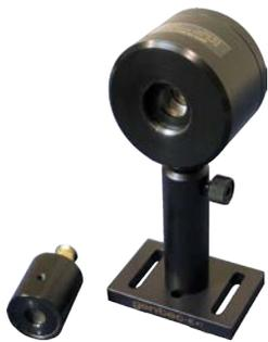
The THZ-WC-13 Accessory is shown prior to installation on our THZ1.5B-MT Probe. The Winston Cone Collar was designed to accommodate THZ windows and is shown with a TPXW window installed. Note that there are two nylon tipped set screws in the collar, that allow adjustment of the position of the Winston Cone to maximize the optical gain.
