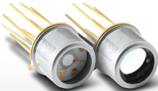
High voltage response Hybrid Pyroelectric Detectors are extremely sensitive thermal detectors. When a thin, LiTaO<sub>3</sub> pyroelectric element is mated to a low noise transimpedance amplifier with a 100 GΩ feedback resistor, the Voltage Responsivity can be as high as 40,000 V/W.
